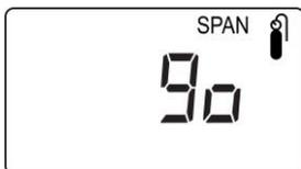
The instrument waits for 10 seconds so that you have time to connect the span gas. Connect the calibration gas adapter to the MeshGuard LEL IR or MeshGuard CO<sub>2</sub> IR, and connect the gas cylinder to the calibration adapter. Start the flow of gas.
