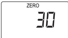
After the countdown reaches 0, the LCD displays “dn,” for “done.” The reading should show 0 (zero). Otherwise, repeat the zero calibration. (LEL reading is shown here.)
