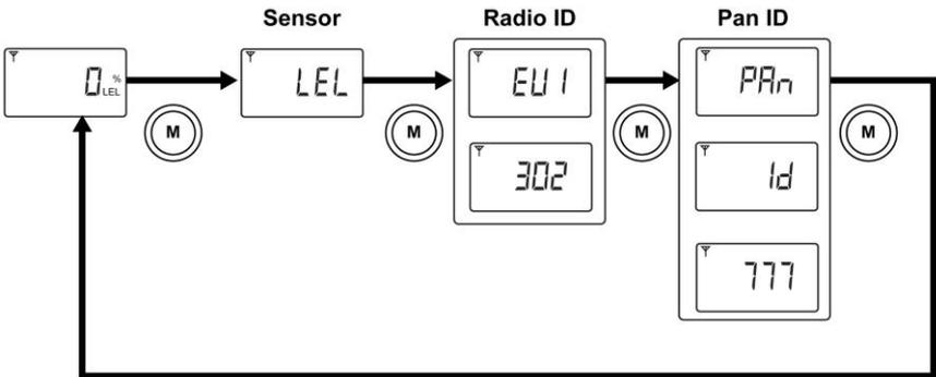
**Note:** The Sensor shows “CO2” in the MeshGuard CO2 IR instead of “LEL.”
