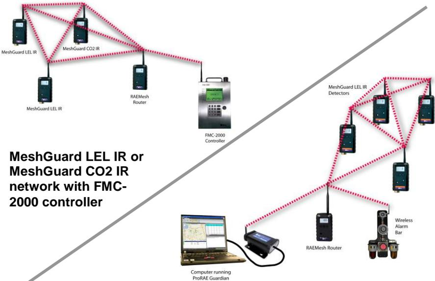
Network with ProRAEGuardian PC controller and Wireless Alarm Bar
