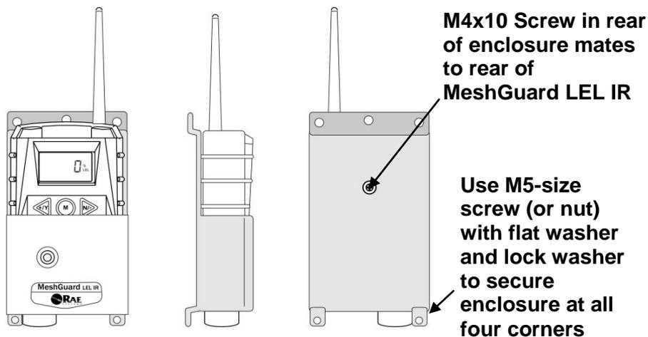
**Front, side, and rear views of the steel enclosure show how the instrument is secured for mounting.**
