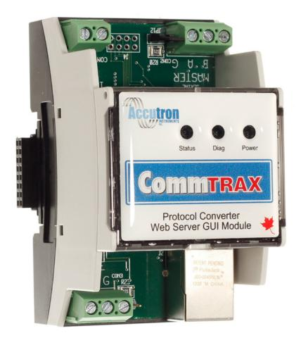
CommTRAX is a compact protocol converter that acts as a server, collecting data from various MODBUS RTU devices and distributing it at a low Bandwidth within a single register package.
